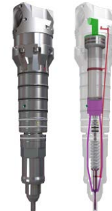
Figure 3 – Picture (left) and cross section (right) of the fuel booster injection valve FBIV used for methanol on the LGI engine. Green lines: Hydraulic oil. Purple lines:
